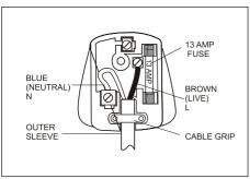
Note: If a moulded plug is fitted and has to be removed take great care in disposing of the plug and severed cable, it must be destroyed to prevent engaging into a socket. If the supply cord is damaged it must be replaced by a service agent or a similarly qualified person in order to avoid hazard.
