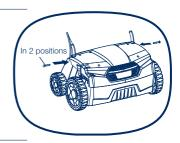
D. Align the middle handle bars to the lower ones. Make sure the holes of the handle bars correspond and secure them with one mounting set on each side.
