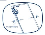
F. Fix the cord with the cord clips to the handle bar.
