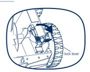
d. Push the scarifying blade cylinder out of the seat.
