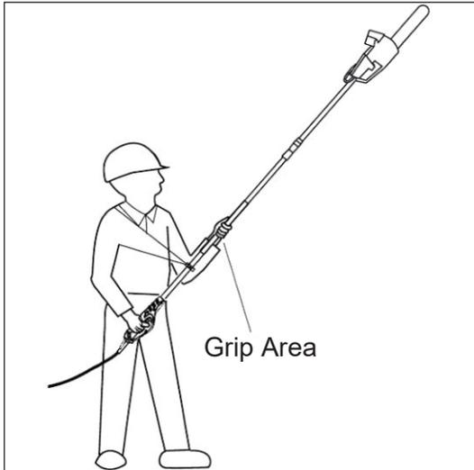
5. When ready to make a cut, press in trigger lock-off button and squeeze trigger. This will turn the pole saw on. Releasing trigger will turn the pole saw off. Make sure saw is running before starting a cut.
