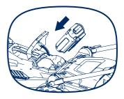
ii. Insert the Safety-Key into assembly hole until you hear a click, then close the battery pack tank cover.
