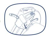
**WARNING:** Before selecting either Vacuum or Blower function ensure that the selector lever operates smoothly and that it is not obstructed by debris from the previous use.
